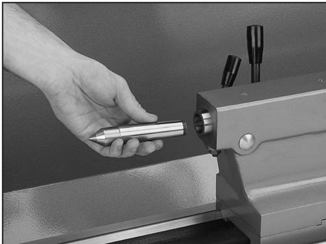
Figure 34. Inserting a dead center in a tailstock.
